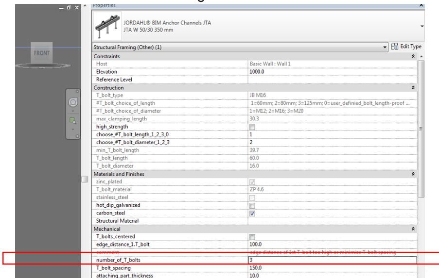
In the above example the selected parameters “edge\_distance\_1.T\_bolt” = 100mm; “number\_of\_T-Bolts”= 3; “T\_Bolt\_spacing”= 150mm for the selected anchor channel JTA W50/30 350mm are not possible, as shown in the highlighted comment. The user might decide to solve this problem by reducing the “edge\_distance\_1.T\_bolt” parameter, or reducing the T-bolt spacing, or selecting a longer anchor channel.
